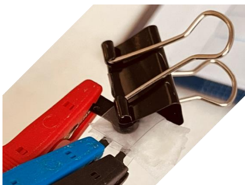
Figure 1 Picture of an electrochemical cell using a paper interface /w sample's solution, screen-printed counter and reference electrodes, and 3d printed PLA/CB working electrode.
